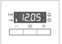
When the time has lapsed, the function indicator will flash, an acoustic signal will sound for 2 minutes and the oven will switch itself off.
